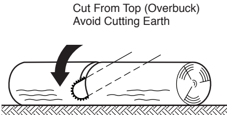
Fig.19 Log Supported Along the Entire Length
