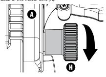
Rotate the entire motor unit (A) until the reference mark on the edge of the motor unit is positioned at the desired head tilt angle (11).
