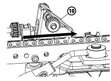
Clamp chain again with the vise handle (13) and sharpen the next cutter.
