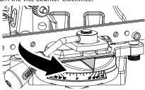
Position the reference mark pointer (17) on the vise by the desired vise rotate angle.
