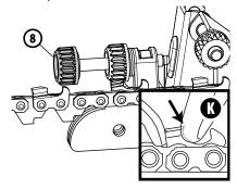
This forward movement corresponds to the quantity of material to be ground from the cutter. The more dull or damaged the cutters, the greater this forward movement should be. For cutters that are not too dull, simply grind a slight amount of material.
