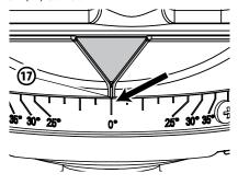
Turn the motor unit (A) to take the reference mark to 80°-75° on the head tilt angle guide plate (11).
