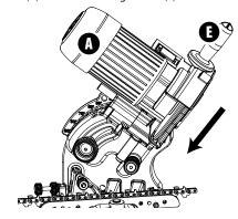
Turn the cutter adjustment knob (8) to move the chain so that the cutter cutting edge skims the grinding wheel (K). The chain should run freely over the vise (14) throughout this procedure but without any clearance.
